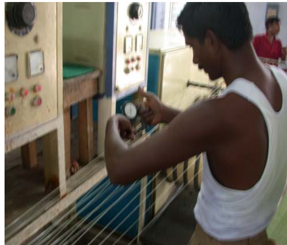
Figure 2 Take the filament and measure the thickness
